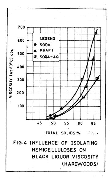
The viscosity of soda-AQ bagasse black liquor at 61% (W/W) solids level is 5200 cps as compared to 800 cps at the same level of solids concentration, after the isolation of hemicelluloses. The same trend was also observed in soda and kraft black liquors from bagasse.
