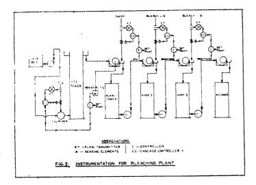
of which will be fed to a controller where predetermined set point is adjusted manually depending on quality of unbleached pulp. The output of controller goes to cascade controller as a new set point. On the other
