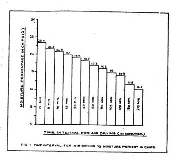
For comparative study of pulping and papermaking chips containing 7, 15, 20 and 25% moisture were taken.
