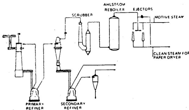
The energy recovery plant in Follum is situated at some distance from the papermill. For this reason, a higher steam pressure is required.
