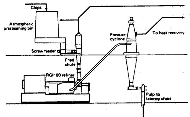
This RGP 60 refiner, which is equipped with an 8 MW (10,800 HP) motor for a production of 100 ADMT/D, incorporates a new design that provides exceptional stability at the very high steam pressure operations that can be of interest in TMP and CTMP manufacture in the future. The RGP 60 refiner is designed for a maximum steam pressure of 9 bar (133 psig.)
