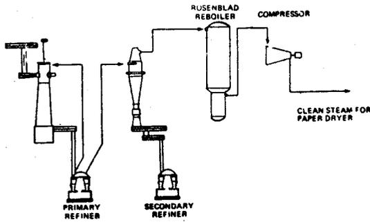
Figure 7. The Follum Mill, Steam Recovery System
