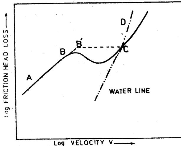
Fig. 6—FIRST DESIGN PROCEDURE BY DUFFY TITCHENER (25)
