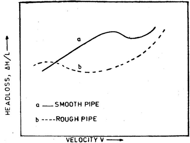
Fig 3—TYPICAL CURVES SHOWING THE EFFECT OF PIPE ROUGHNESS FOR FLOW OF SAME PULP SUSPENSION.
