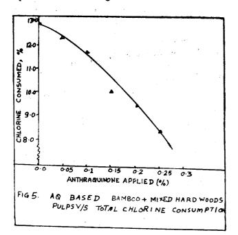
The fibre classification of bleached anthraquinone based bamboo+mixed hard woods (70:30) pulps was carried out in a Bauer Mc nett classifier. The fibre retention on different meshes is tabulated in Table-5. The anthraquinone based bleached pulps were also beaten in a valley beater at 45°SR and the physical strength properties of the sheets like tensile Index, Burst Index and Tear Index versus anthraquinone dosages applied are shown in figure-6.
