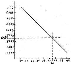
WATER REMOVED FOR 100 TPD PRODUCTION AT DIFFERENT SHEET DRYNESS PER HOUR GRAPH NO.1
