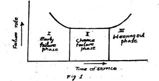
In the early failure phase I, the equipment being new, the failure rate comes down. At this stage the manufacturer's recommendation carries an important weight in deciding the requirement of spares. The second stage is often characterised by a constant failure rate and here only chance failures occur. The third part is characterised by an increasing failure rate and it is the period during which components fail because they are worn out.
