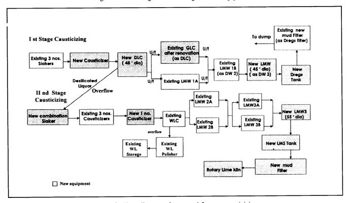
Figure-2: Flow diagram of proposed 2-stage causticising process.
