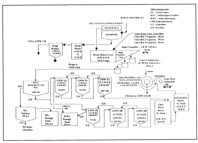
Figure-1: Flow diagram of existing causticising process.
