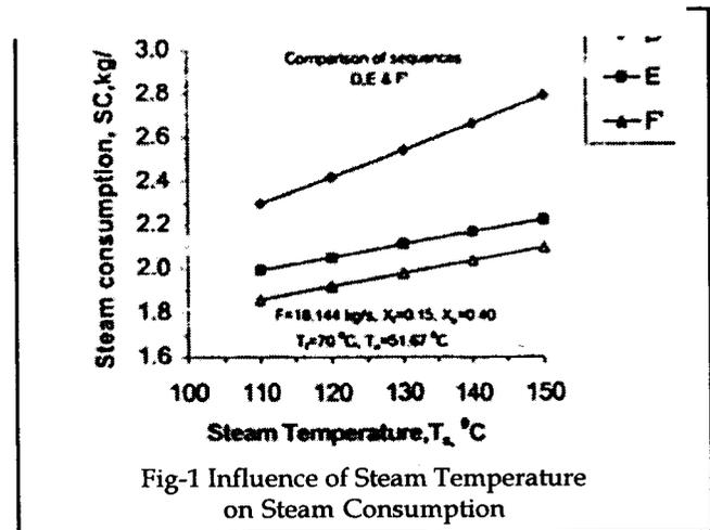
Fig-1 Influence of Steam Temperature on Steam Consumption
