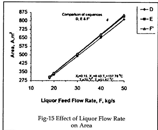
Fig-15 Effect of Liquor Flow Rate on Area
