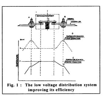
maintenance procedures must include regular inspection / tightening of these termination.
