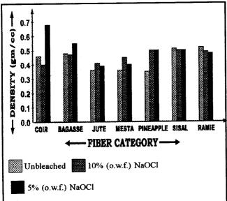
Fig. 2 Graph showing the Density (gm/cc) of the papers made from different fibre types under different conditions of bleaching.
