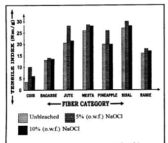
Fig. 3 Graph showing the tensile index (Nm/lg) of the papers made from the different fibre types under different conditions of bleaching
