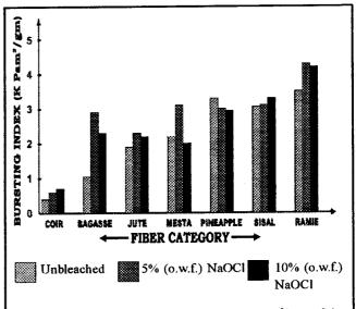
Fig. 4: Graph showing the bursting index (K Pam²/gm) of the papers made from different fibre types under different conditions of bleaching.
