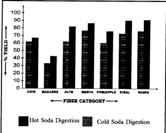
Fig. 1 Graph showing the pulping characteristics of the different fibre wastes in terms of percentage yield of the pulp
