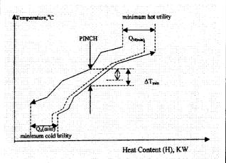
Fig. 5 Energy targets and "the pinch" with Composite Curves
