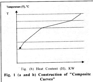
being done within the system. In a system where only required heating and cooling are maintained, the heat flows across the Pinch is zero. This system is identified as a system where utility targets are achieved very close to optimal conditions (Fig. 3a) where external heating is done in excess over the minimum possible requirement of the processes. The heat balance shows a heat flow across the Pinch and therefore an excess external cooling is required (Fig. 3b).
