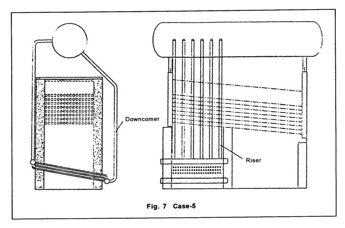
one of the drums, as the NRV was defective. It is possible that flow reversal was taking place in the downcomer in the drum where the NRV was not functioning. The NRV at each steam drum inlet was removed and a common NRV was provided in the feed line. Also a feed distributor was added in each drum to distribute the water to downcomer area. This way the flow reversal in the downcomer was eliminated and the failures stopped.
