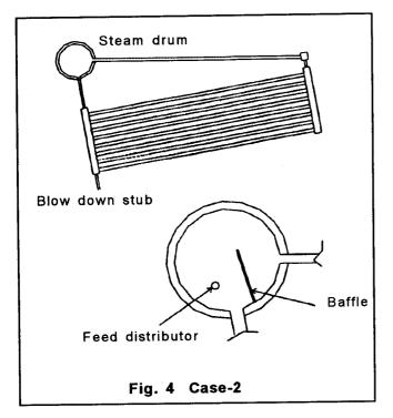
way that heat flux and heat duties in various circuits are more or less same. If tubes are inclined close to horizontal, the steam separation would take place leading to overheating of tubes.
