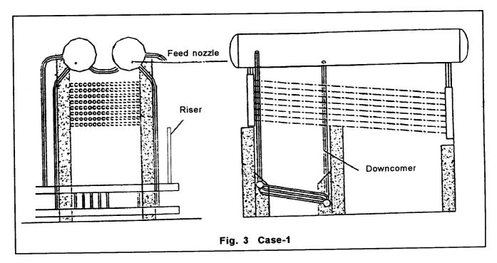
heated evaporator section to poorly heated evaporator section. It would be necessary to separate the poorly heated section if it lies in paralel to well heated section. The downcomers and risers are to be arranged separately so that the reliable circulation can be ensured. This principle is called sectionalizing for reliable circulation. The inlet headers/outlet headers shall be partitioned for this purpose. However, it is desirable to arrange the evaporative surface in such a
