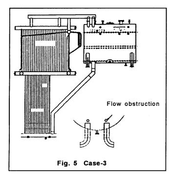
also form part of the natural circulation circuit. The baffles are arranged in such a way that the steam would rise easily to the steam space without much resistance. High - pressure drop in the drum internals will retard the flow through evaporator tubes.
