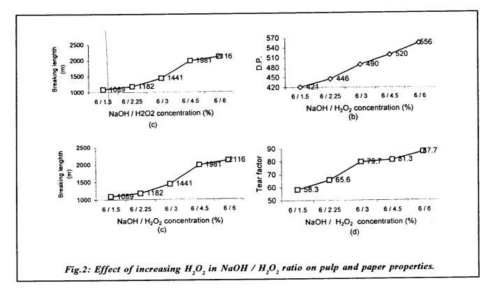
and 2116 m at 6%  $H_2O_2$ . From the above results, it could be concluded that with increasing  $H_2O_2$  in NaOH/ $H_2O_2$ ratio, the best pulping results can be obtained with respect to screened yield, reject chemical and physical properties of pulps.
