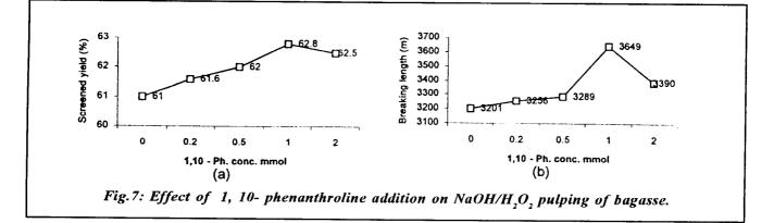
and then decreases with increasing 1,10-phenanthroline concentration to 2 mmol. From these results, it can be concluded that the addition of 1 mmol 1,10phenanthroline during the alkaline hydrogen peroxide pulping of bagasse is considered as the best concentration at which the efficiency of the delignification processes increases.
