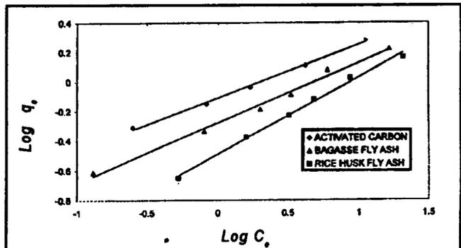
Fig. 12: Freundlich Isotherm for removal of 2,4 dichlorophenol by different adsorbents
