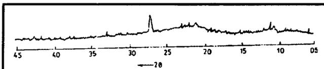
Fig. 6: X-ray diffraction pattern of rice ash husk
