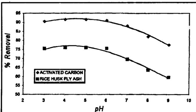
Fig. 9: Effect of pH on removal of 2,4-dichlorophenol
