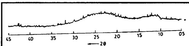
Fig. 7: X-ray diffraction pattern of bagasse fly ash
