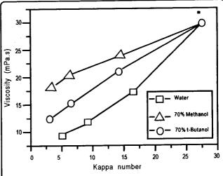
Figure 3. The Lignin-Cellulose Selectivity During Ozonation of Hemlock Kraft Pulp in Different Solvent Systems
