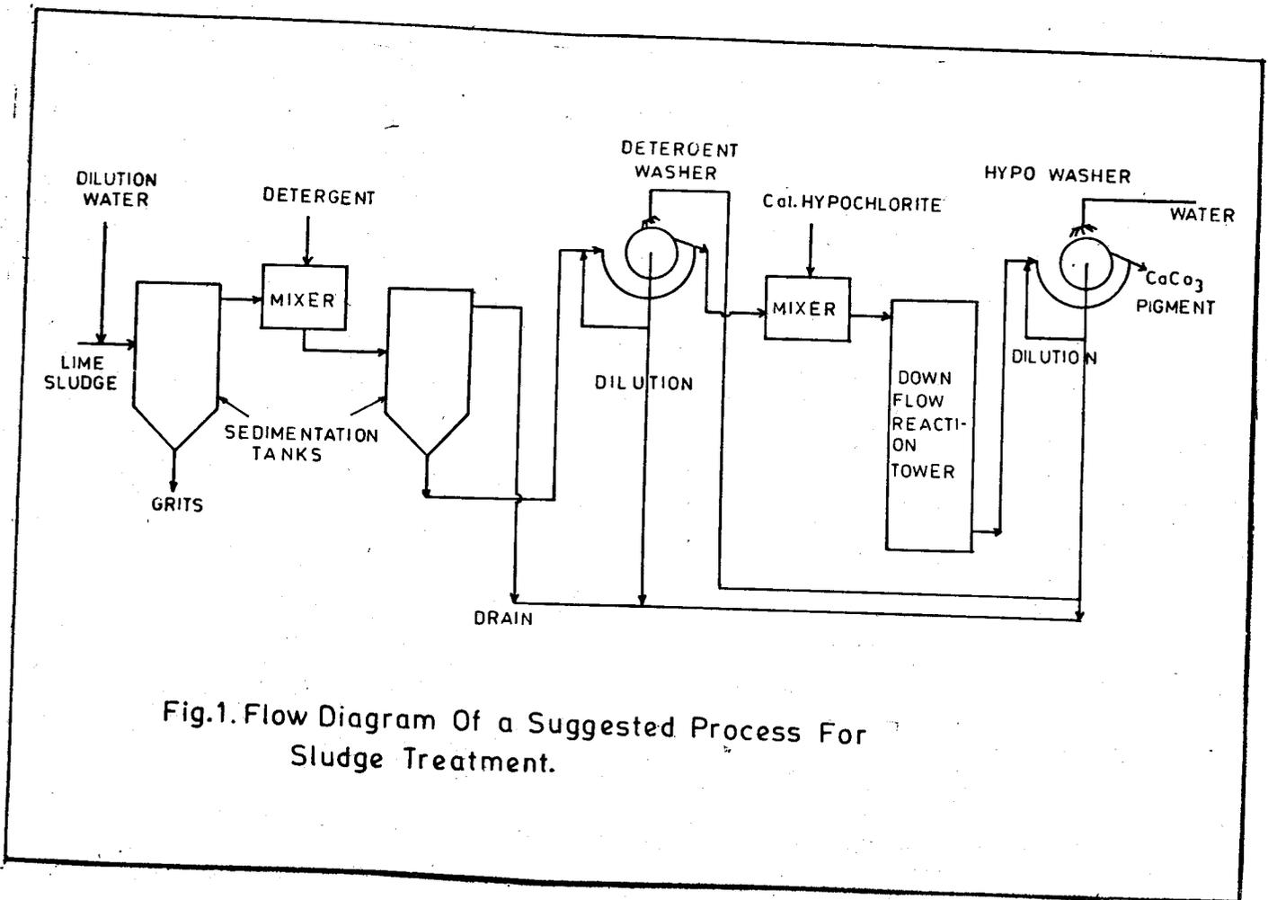
Fig.1. Flow Diagram Of a Suggested Process For Sludge Treatment.
