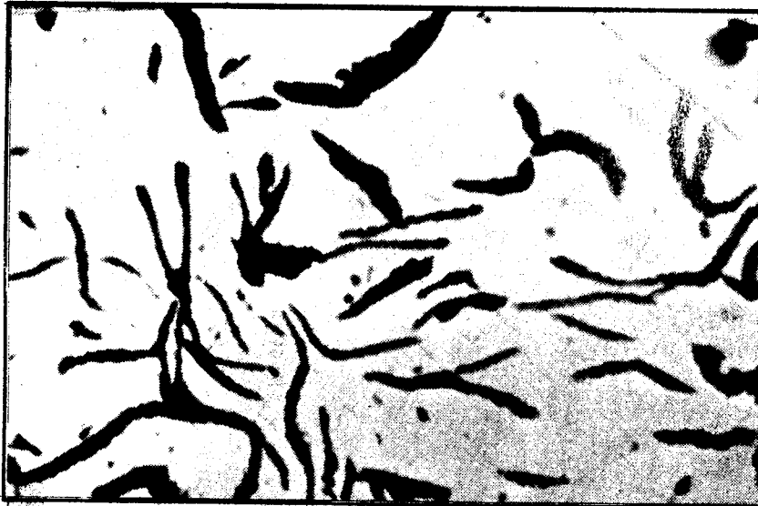
Fig. 7: An un-etched micrograph showing the flake morphology of dryer shell material, magnification = 100 X.
