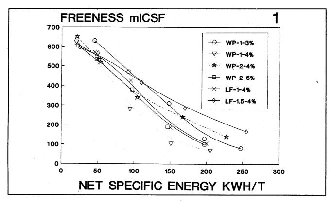
2000 Ws/km SEL as the fibre is cut compared to that of pulp refined with 1000 Ws/km SEL where it is otherwise as the fibrillation of the fibre takes place.
