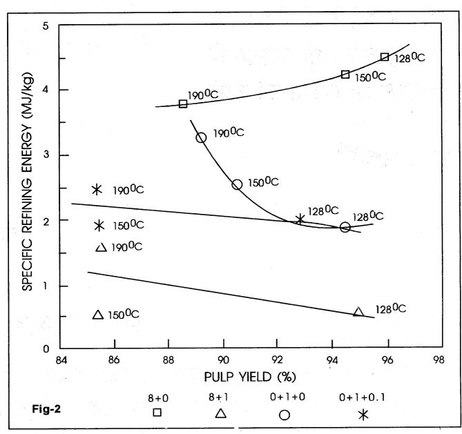
increases from 1.65 to 3.3 MJ/kg (i.e. an increase of 100%) with the rise of cooking temperature from 128 to 190 °C. The pulp yield decrease from 94.5% at 128 °C to 89.2% at 190 °C.
