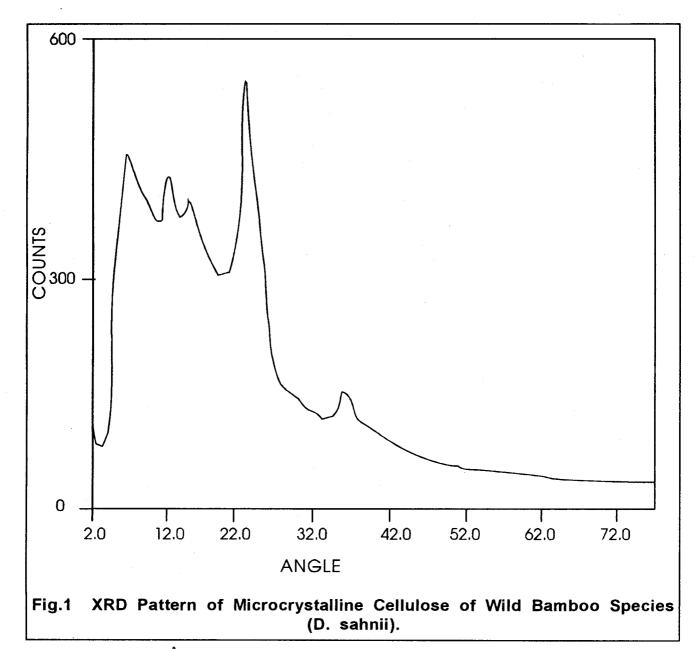
of nitric acid but it effects the yield. The crystallinity percentage was found to be 28%. The average value of crystallite size in (002) plane direction was found to be 8.2 nm (corresponding to 10 cellulose unit cells) and it was 18.8 nm (corresponding to 18 cellulose unit cells) in (040) plane direction. It can be concluded from the present investigation that microcrystalline callulose obtained from this bamboo species is found suitable for industrial use.
