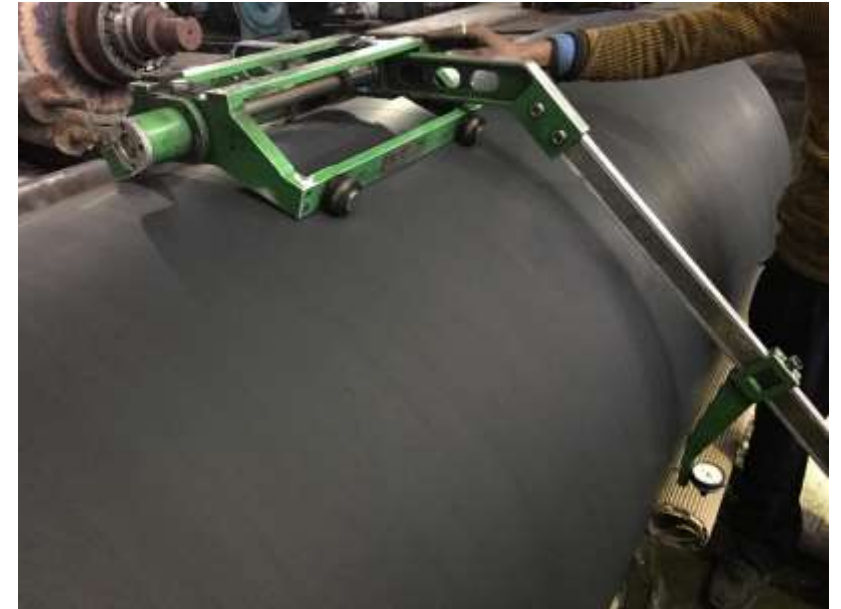
CHECKING CAMBER ON ROLL WITH TROLLEY
