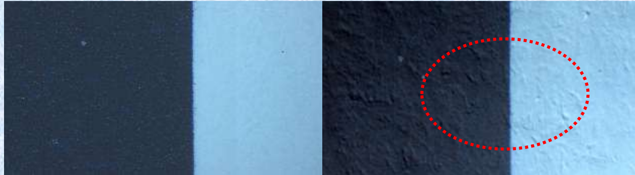
Good Sample – Uniform Surface Topography Bad Sample – Non Uniform Surface Topography
