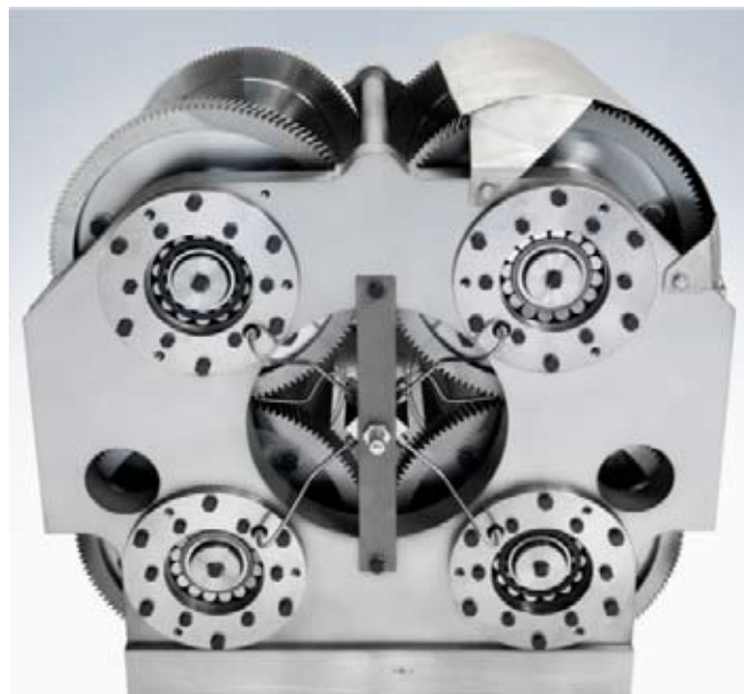
Fig: 2, DuoShake: Improves fiber orientation & formation
