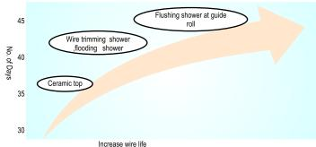
In PM-3 couch trimming was getting carried along with the wire, as a result of which edges of the wire was getting worn out.
