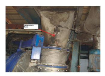
In the disperser section, the equalizing screw got jammed due to the pulp accumulation in the discharge chute. A paddle was fitted to equalizing screw for evenly distribution of the pulp & high pressure shower nozzle was fitted in the discharge chute to avoid the pulp accumulation. It is operated from DCS with a timer. If this shower opens continuously, it will reduce the disperser inlet consistency. So it was connected to DCS & operates with timer after a certain interval for a few second.
