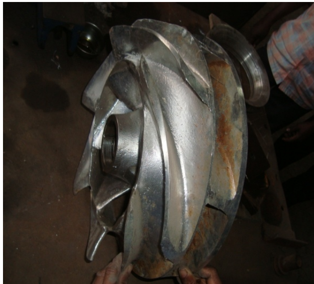
6 vane staggered old Semi open impeller
