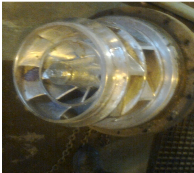
7 Vane staggered new Closed impeller
