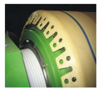
and a new blanket is slid on from the frontside end. Support systems for the shoe module during this period are built into the unit, and a frame for holding the blanket to the right shape and supporting the front of the roll is provided. Belt change time is of the order of 3 hours.
