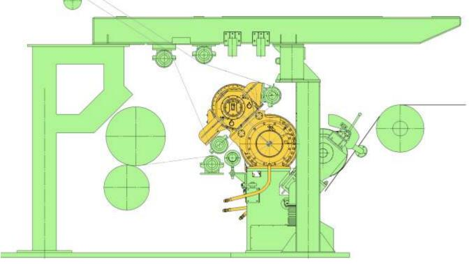
the circular heads make the blanket follow a completely circular path. Over the shoe width the path is not fully circular, having of course the concave depression due to the nip. In the transition zone between these areas (outboard of the shoe width at front and back) the blanket undergoes a degree of flexure that is the source of eventual hardening.
