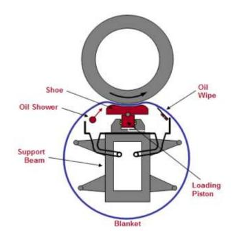
circular heads at each end. These heads, and the blanket attached, are the only rotating part of the assembly, and are mounted on large bearings on the support beam journals.
