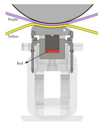
In this diagram, the blanket is shown in yellow. The purple represents the combination of one or two press felts, together with the sheet. In the case of a single felted press, the sheet would be between the felt and the opposing roll. The sheet is never run in direct contact with the blanket.
