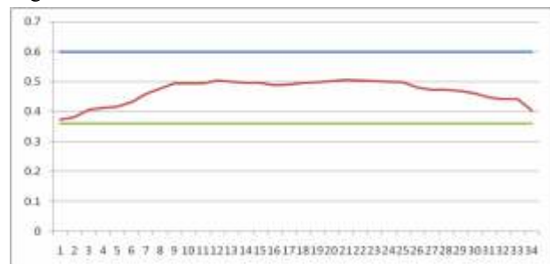
Fig.2: Wear pattern of wire mounted with new suction box tops
