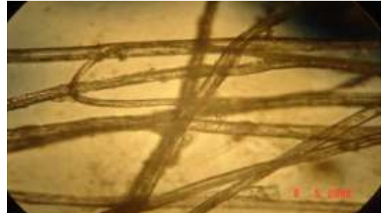
Fig. 8. Fibers beaten in a beater (1.30hr)
