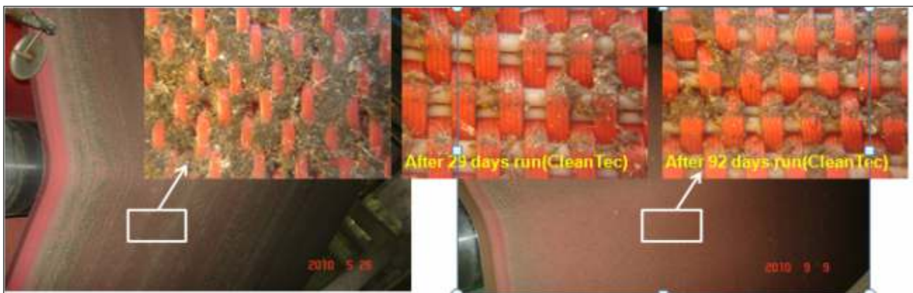
After 26 days run(Dongil, 150cfm) Removed and HP water gun cleaning: every month
