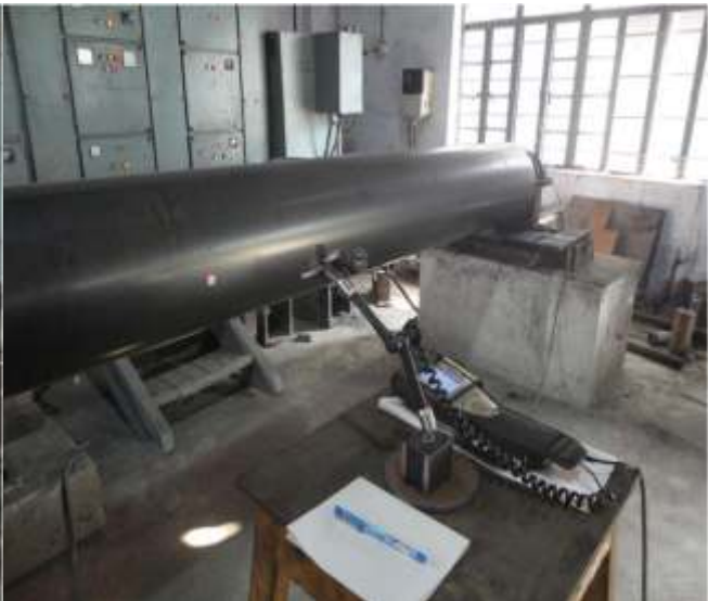
(Dual plane balancing is done at both side of roll by a trigger and Vibration sensor, connected to a vibration logger having software of dual place balancing)
