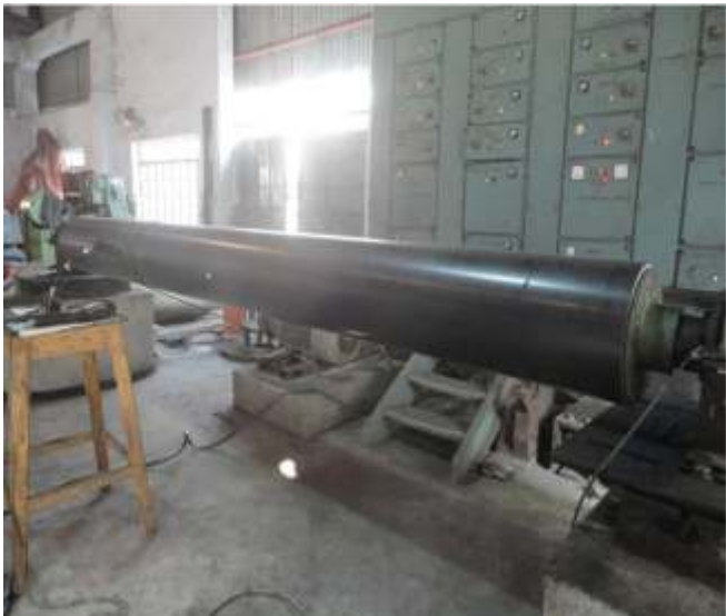
(Dual plane balancing is done at both side of roll by a trigger and Vibration sensor, connected to a vibration logger having software of dual place balancing)
