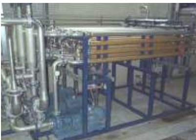
Figure 6: Side view Membrane Unit
