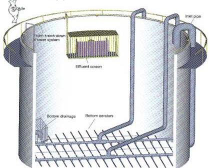
kept in parallel, equipped with surface Aeration system and Moving Bed Bio-Film with diffusers aeration system for biological degradation of the waste.
