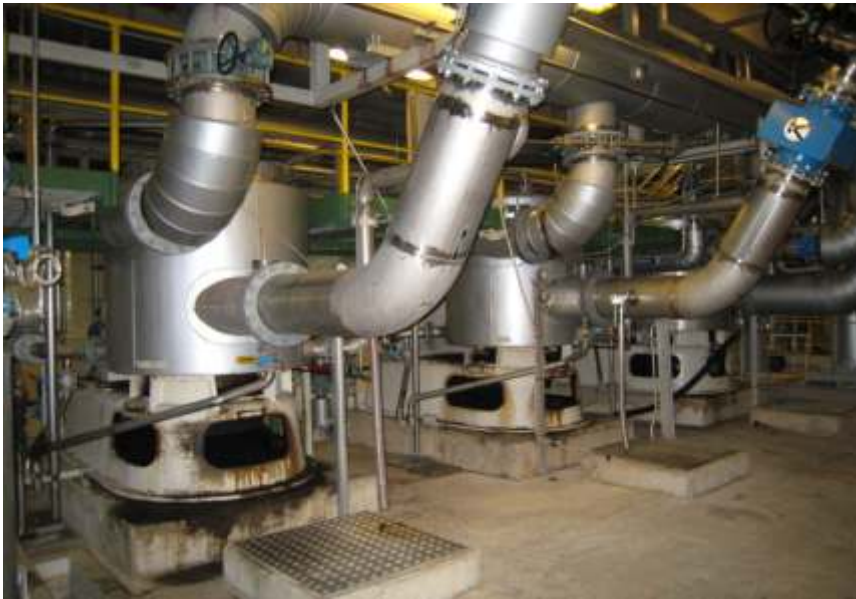
Figure 2. The M800 Centrisorter pressure screen with the AFT GHC™ Rotor and AFT MacroFlow™ Cylinder is shown in the centre of the photo. The M800 Centrisorter fitted with competitor components is on the left.
