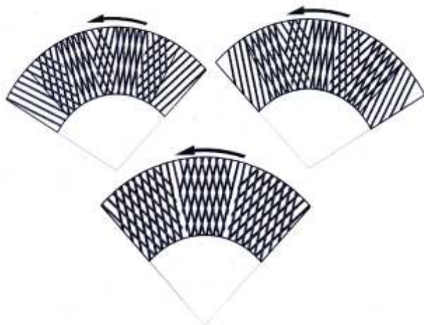
Changing Crossing Angles in Parallel Bar design
