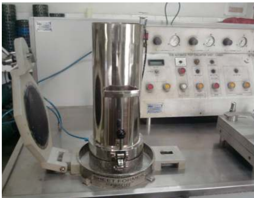
(Fig -1 : Laboratory semi automatic hand sheet former Model FBI 7, Fibre tech Instruments, Roorkee).
