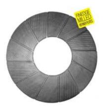
technology to provide the maximum uniformity in the refining zone. Milled blanks are cast in own foundry as a solid piece to provide uniform hardness through out. The plates will wear uniformly over time, and with the zero draft angle on the bar, hydraulics are maintained longer. The Parason precision CNC milling manufacturing provides accurate groove width, which allows finer bar to optimize low intensity applications. Plate life is also maximized by re-grooving which allows 2-3 life cycles.
