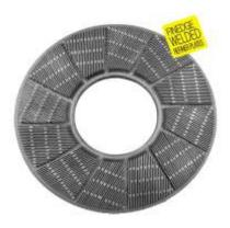
Special Features: Narrow bar width from 1.6mm, bar width range 1.6,2.0,2.5mm on wards, high cutting edge length, zero draft angle on the bar, More bar height more life & special metallurgy.
