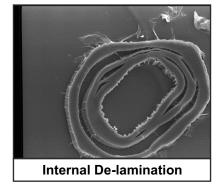
Forces applied on the fiber by the bars of Stator & Rotor in Refiner cause fibrils to move relative to each other, breaking bonds and thus causing fiber de-lamination.
