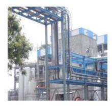
Delignification followed by ECF Bleaching with D0/EOP/D1 sequence to meet brightness level of 87+.
