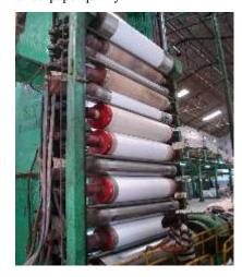
The second aspect was of roll performance. For the same, it was decided to run the calender bypassing all paper rolls, and having a close look on roll condition. For this, during every reel change, the temperature of cotton rolls was recorded using a non-contact type pyrometer. The increase in temperature was only 5-6°C compared to that when paper rolls were in operation. This problem was solved by the method describe later in this paper.
