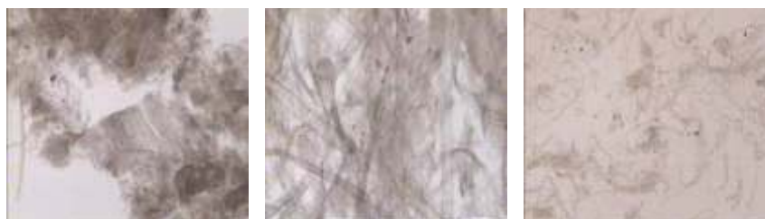
Fig.2 The configuration of collagenous fiber with refining after acid-hydrolysis
