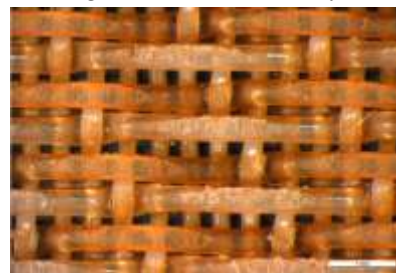
Figure 12: The condition of the MultiForm HC after running a new record life on a DuoFormer Base top.
