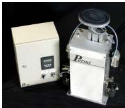
Figure 1 Remote control box and measuring head
