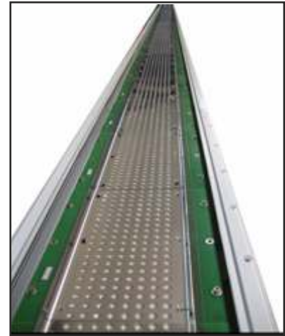
Fig.3: LED light beam for a 9m wide web
