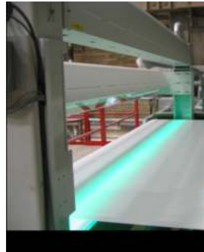
Fig4: High angle reflection and transmission illumination on a board machine
