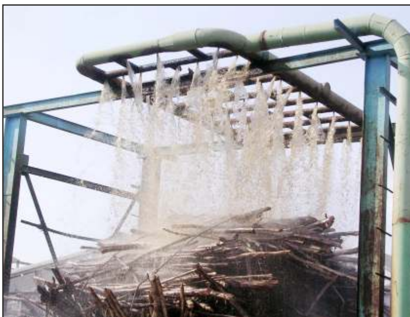
PHOTO 1 USING OF TREATED WATER FOR WOODEN LOG WASHING IN CHIPPER HOUSE
