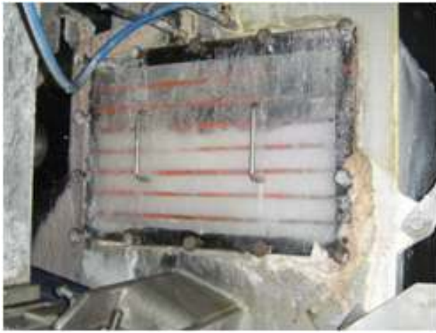
The sight glass of top former was kept clean even after running with 17 days with Amox
