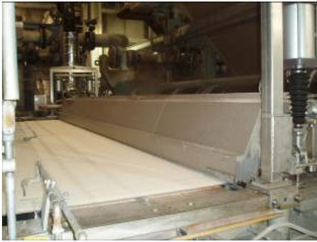
Figure 2a: New Steambox with no Steam Spillage
