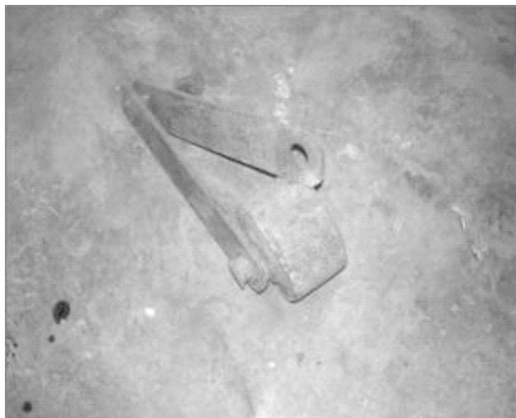
Fig. 6 Worn out hammer
