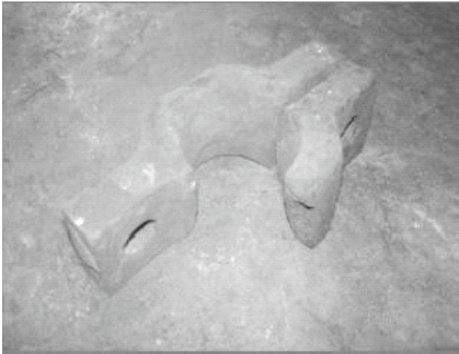
Fig.7 Worn out Plummer block
