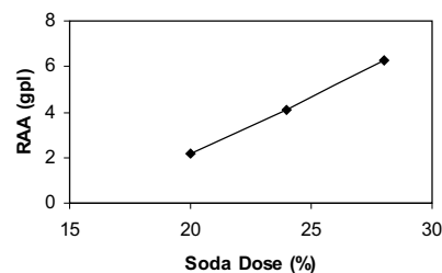
Figure 3 : Effect of soda dose on residual active alkali (Soda-AQ pulping)
